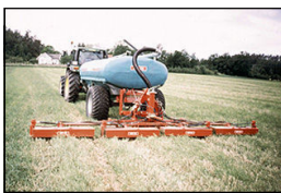
A tank fertilizer truck trenches urine into the soil for grain crops in Sweden
